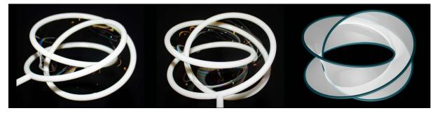
(a) Soap film on wireframe (b) Oriented soap film on wireframe (c) Simulated soap film surface
