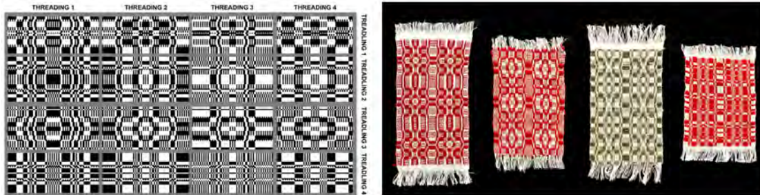
Figure 6: The first example of bringing the code to fruition with physical samples. Left: A grid of 4 expanded threading options. Right: The woven samples from threading 2.
