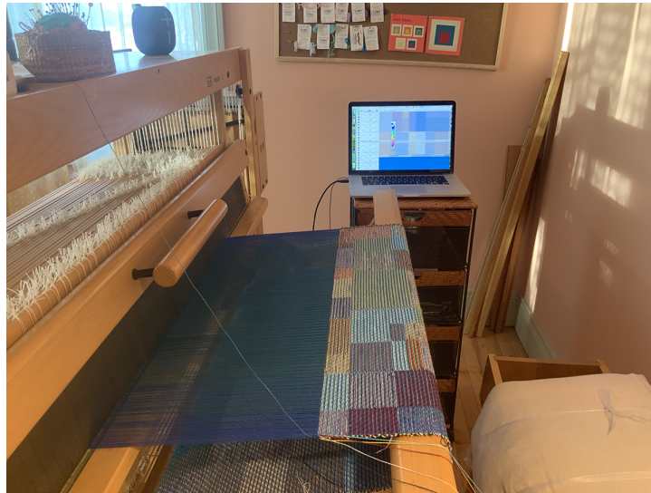
Figure 4: The 32-shaft computer-aided loom in the author’s studio. Photo credit: Patricia Bentley.
