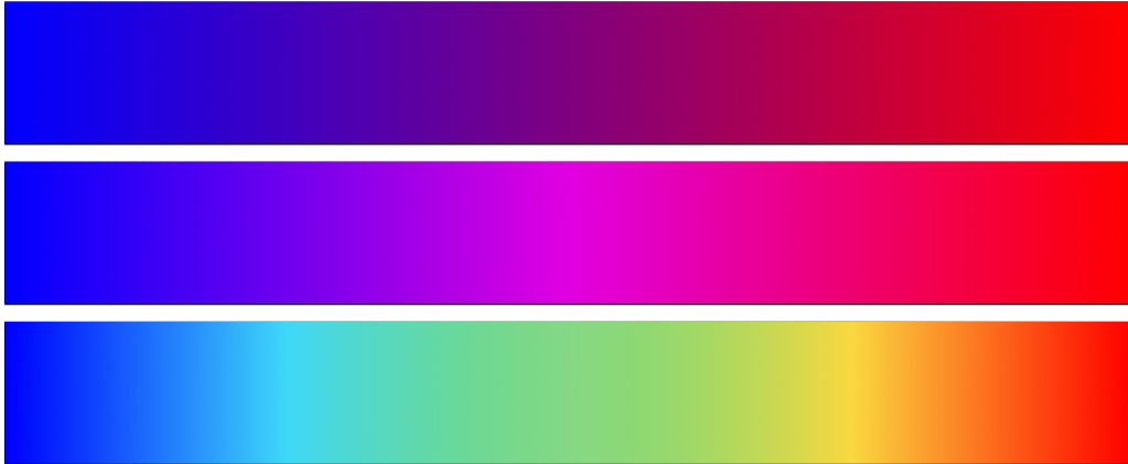
Figure 3: Example of a linear gradients. RGB space(top). HSL space: anti-clock-wise (middle) and clock-wise (bottom).
