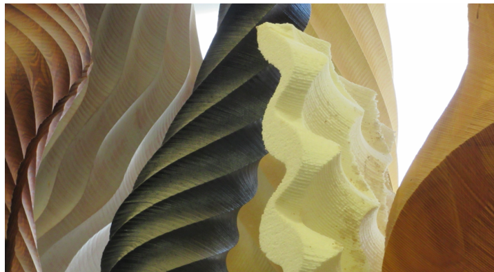
Figure 3: The flutes are formed by the operator's successive plunge cuts.
