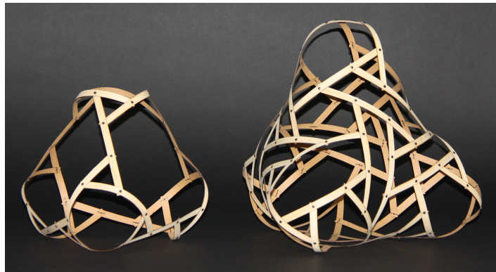
Figure 5: Reciprocal structures based on the truncated tetrahedron. The conventional reciprocal structure with 18 strips (left) and the paired strip reciprocal structure with 36 strips (right).
