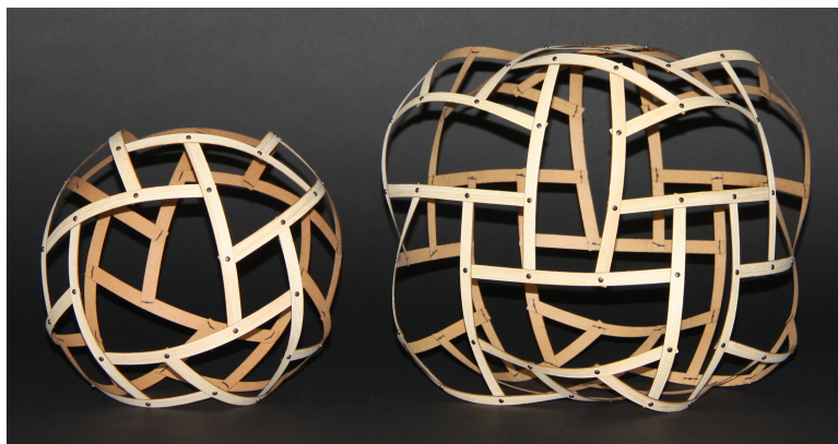
Figure 6: Reciprocal structures based on the cuboctahedron. The conventional reciprocal structure with 24 strips (left) and the paired strip reciprocal structure with 48 strips (right).
