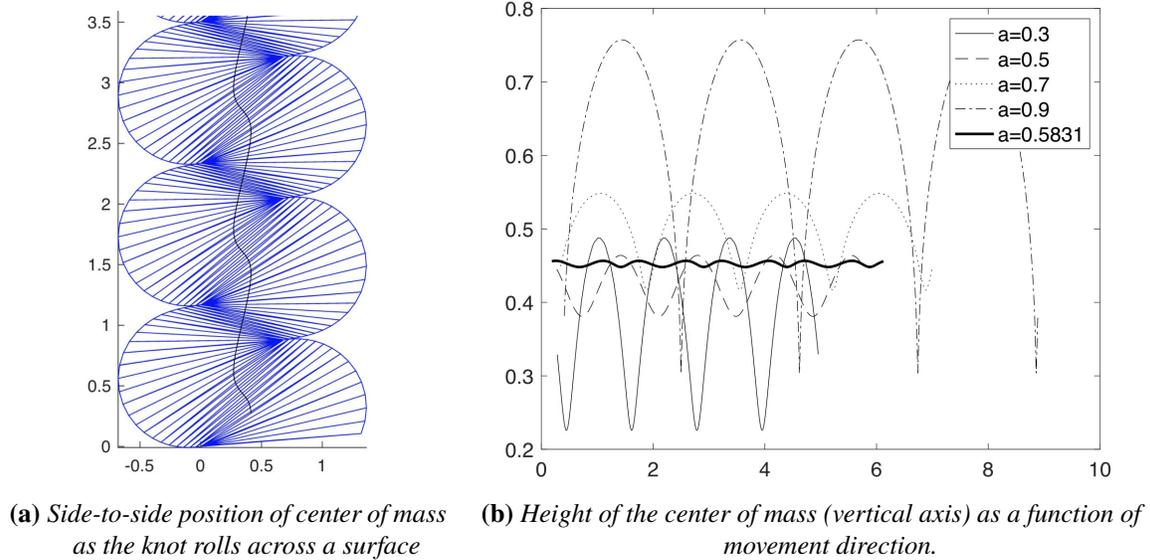
**Figure 3:** Center of mass movement from side to side for one Morton's knot with  $a = 0.3$  and  $R + r = 1$  (a), and up and down for many Morton's knots with differing values of  $a$  and  $R + r = 1$  (b).
