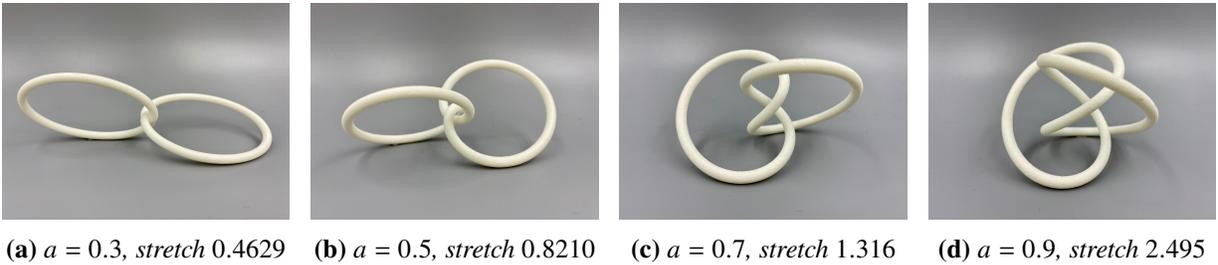
**Figure 4:** 3d printed stretched Morton knots with  $R + r = 1$  and various values of  $a$ .
