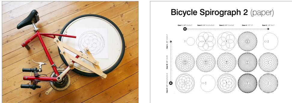
Figure 5: Bicycle Spirograph 2 (Paper) , 2017, and the 15 patterns that can be drawn with its 15 gears.
