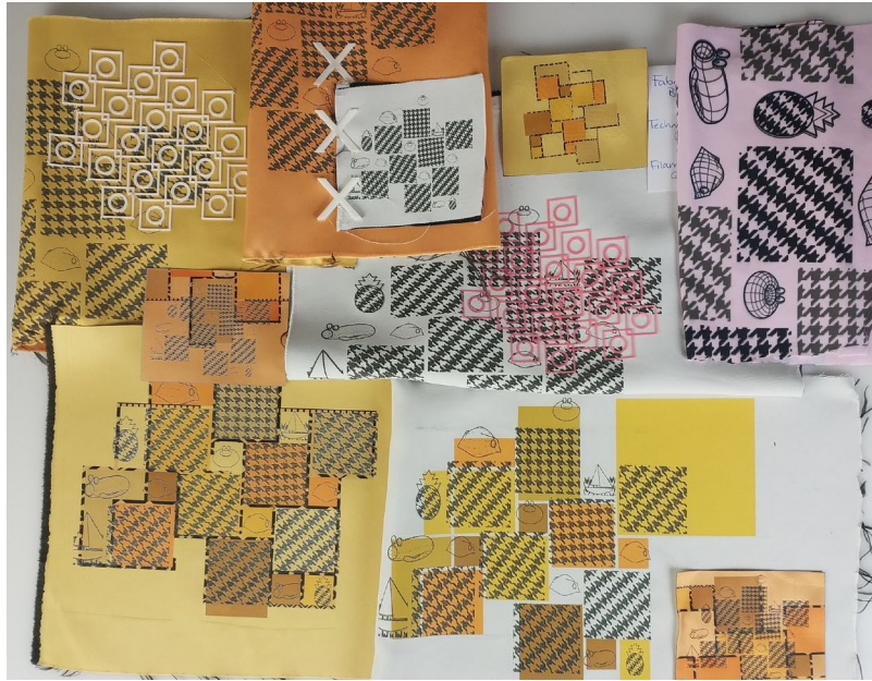
Figure 10: Experimental print samples. Top row (from left to right): laser engraving with 3D printed TPU on top, engraving with 3D printed TPU to connect (engraved) patch, (small) sublimation print, monochrome sublimation print on pink jersey. Middle row: engraving and sublimation printing, engraving with 3D printed thermochromic filament. Lower row, from left to right: engraving with sublimation on top, engraving with partial sublimation on top, (small) engraving with sublimation on top.
