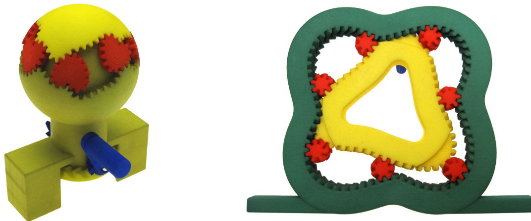
Figure 9: a) Valentine Gear Sphere , b) Captured Gears , both 3D printed at Materialise.
