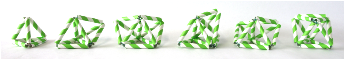
Figure 8: All nonisomorphic minimally rigid graphs in 3D up to 6 vertices constructed using straws and filament.
