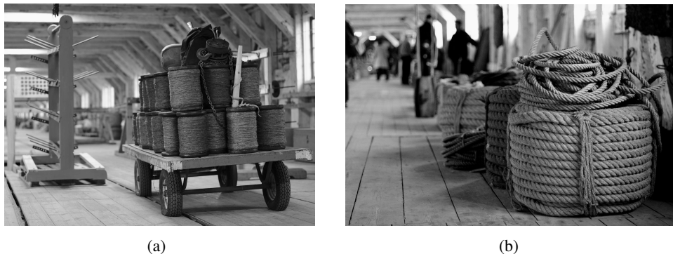
Figure 2: Examples of different rope materials at the Naval Rope-walk on the Island of Lindholm in Karlskrona, Sweden: (a) yarn made of hemp and (b) modern produced (pre-1960) Coir rope. Photographed by A. Åström 2015-10-10 and 2010-10-09 with permission from the museum.
