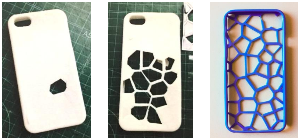
Figure 4: Different stages in the making of a case for mobile phone based on a Voronoi diagram.
