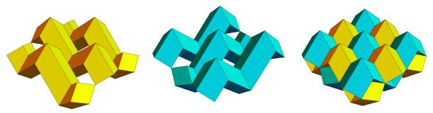
**Figure 9**: Weaving two orthogonal sets (left, middle) of three  $90^{\circ}\sqrt{2}$ -rhombic zigzags into a tight fabric (right)
