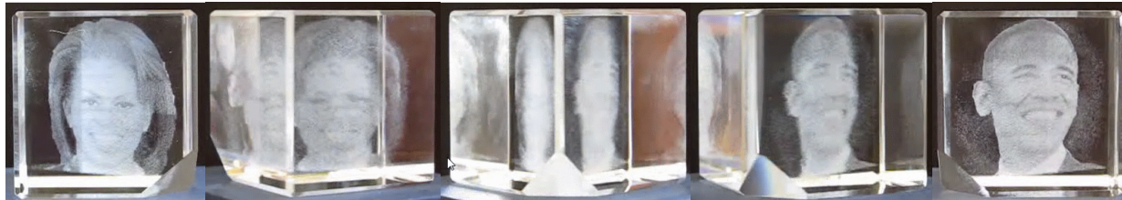
Figure 1 : 3D-dithering of two 2D images of the Obamas (left and right), etched in one 3D glass cube.
