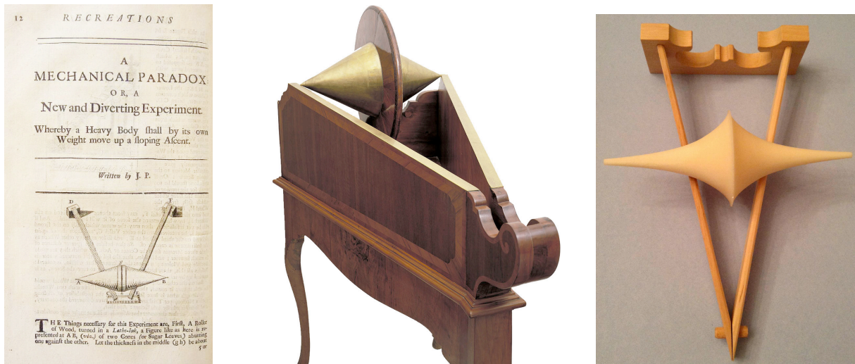
Figures 5a (l), b (c.) & c (r.): (a) The original 1694 description of “A Mechanical Paradox” employing a double cone; (b) 18 th century wood and brass version displayed in the Museo Galileo in Florence, Italy; (c) Our plastic rapid prototype pseudosphere in its equilibrium position on a wooden double ramp.
