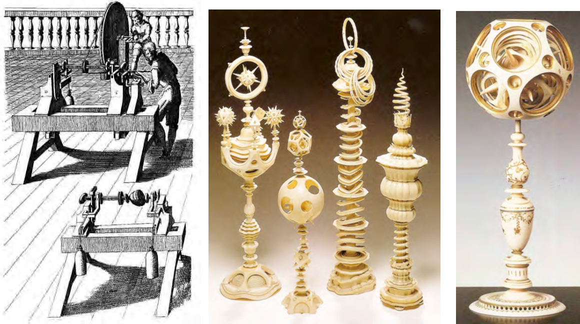
Figure 8 a, b, c: On the left is an engraving of an ornamental turning engine from about 1600 AD. In the middle and at right are examples of ivory ornamental turnings produced between about 1560 and 1590 of the kind that are in the Grünes Gewölbe (Green Vault) museum in Dresden, Germany.
