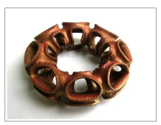
**Figure 1**: Yutu Liu's 3D printed physical Inout sculpture. This sculpture is 3D printed using Dimension SST and made from ABS plastic. It is painted with gold color spray paint.
