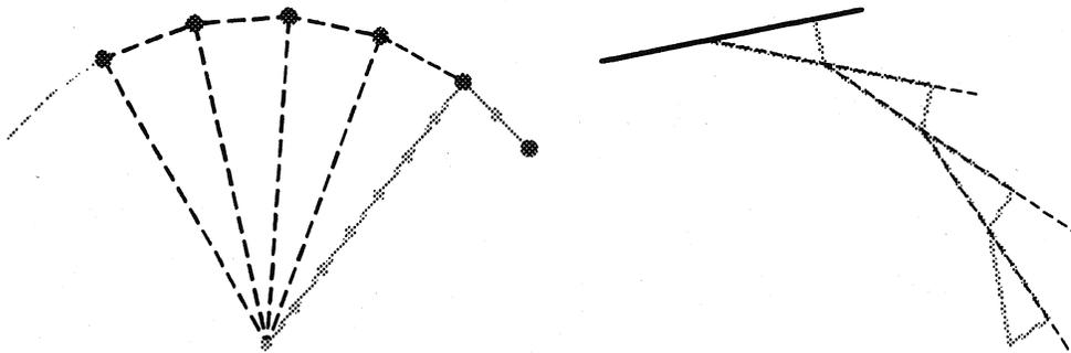
**Plumbs.** A weighted line is the universal measure of verticality. Early versions were weighted with stone, and later lead, thus the name plumb line. Roman and Egyptian practice provide clues as to how the plumbed line may have been used by Neolithic builders. One function was that of a level or inclinometer (see diagram below). The most frequent application of the plumbed line, though, was as a sighting device.
