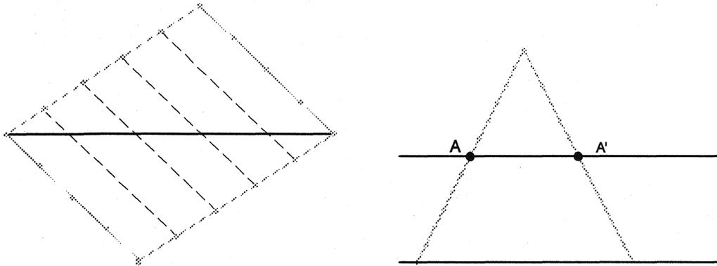
**Arc Layout.** One can rarely scribe an arc when surveying in the field. Grass and rocky ground are not conducive to accurate scribing. Consequently surveyors typically describe an arc with a series of equally spaced stakes. This is also the method used today for forming curved concrete walks, where stakes are interpolated with flexible metal strips to achieve curvature.
